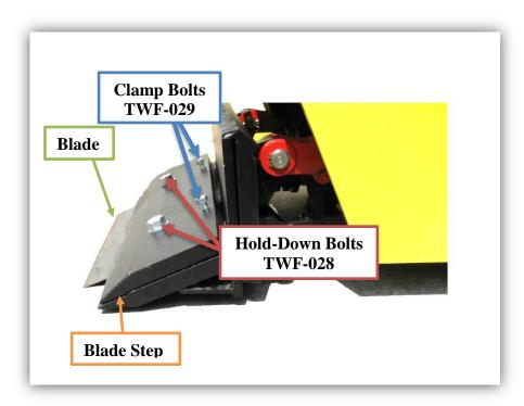
**Clamp Bolts** with your wrench. Lower the blade and resume scraping. With a little practice, you should be able to change the blades in 15 seconds. Dull blades may be sharpened and reused many times.
